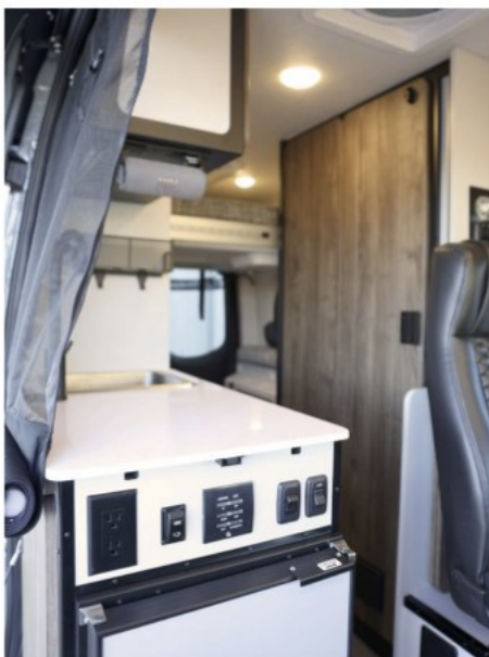
The GH1's galley has a 3.1-cubic-foot refrigerator and a portable induction cooktop.
