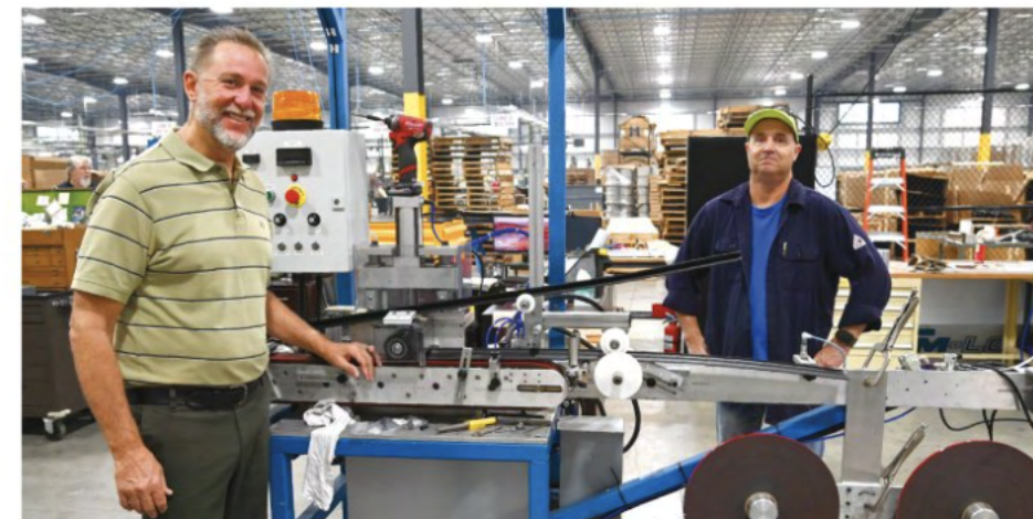
[L to R] Whitener and Mike Oltman, maintenance associate, test the taping machine to ensure the machine is accurately applying tape to Trim-Lok products.
