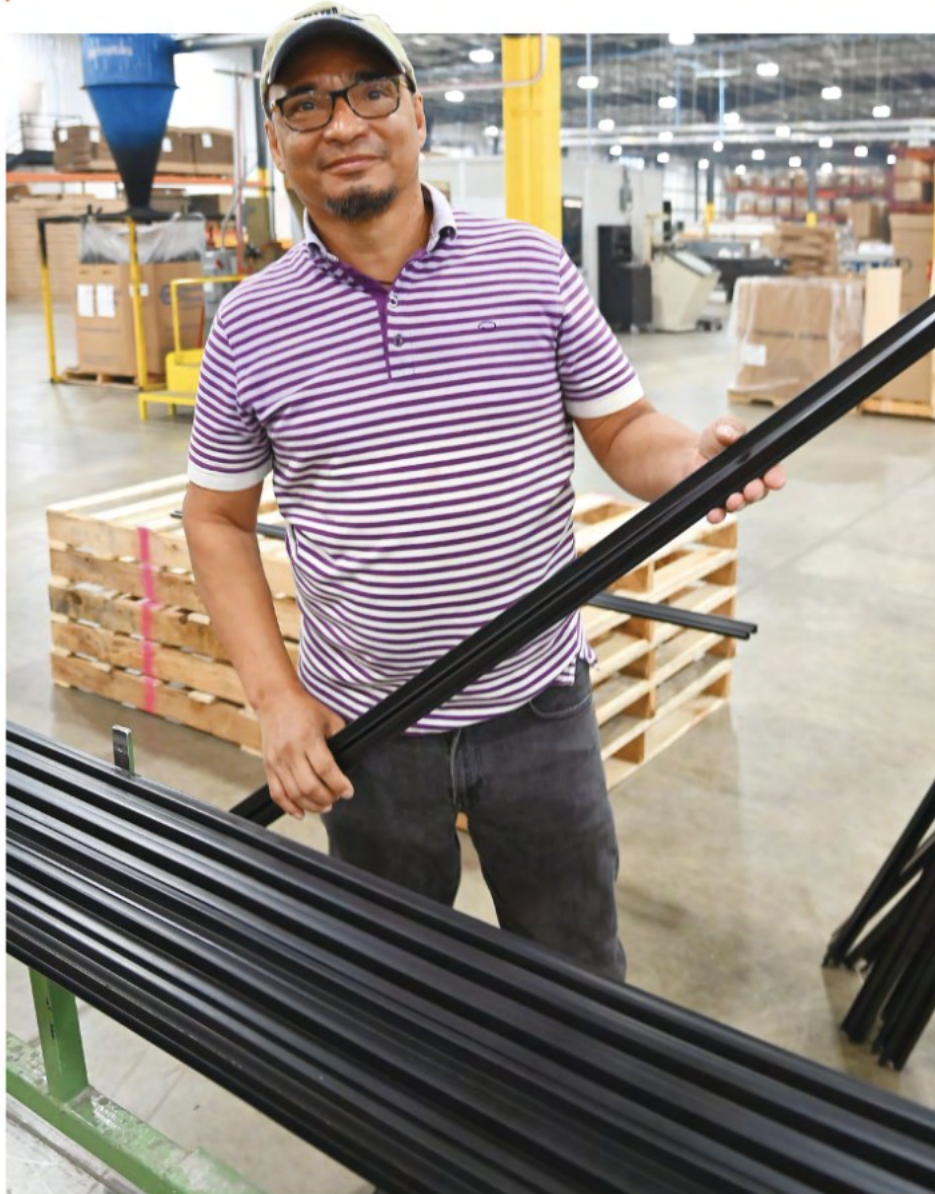
Production Supervisor Carlos Fuentes collects RV trim. The plastic pieces pictured replaced aluminum parts Trim-Lok previously made.
