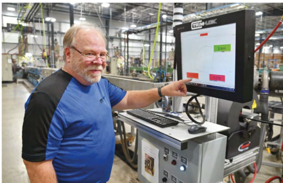
Quality Manager Jim McVay uses a digital comparator to inspect Trim-Lok parts.
