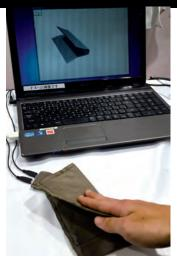
There are three weave versions: plain weave detects bending, satin weave detects twisting, and twill weave detects shear and 3-D motion, as well as bending and twisting.
