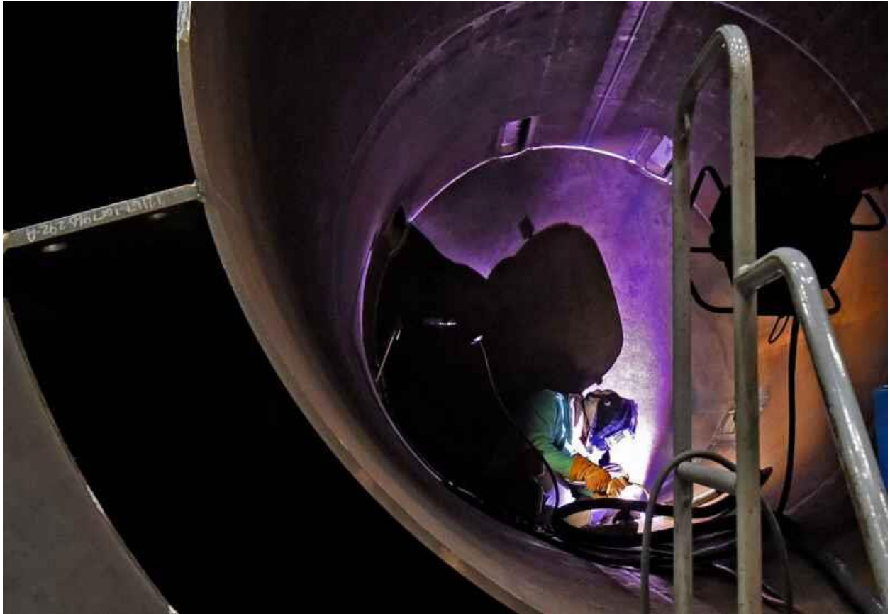
A Holtec associate welding the interior of a HI-Storm overpack dry fuel storage system at Holtec in Camden, N.J. (April Saul)
