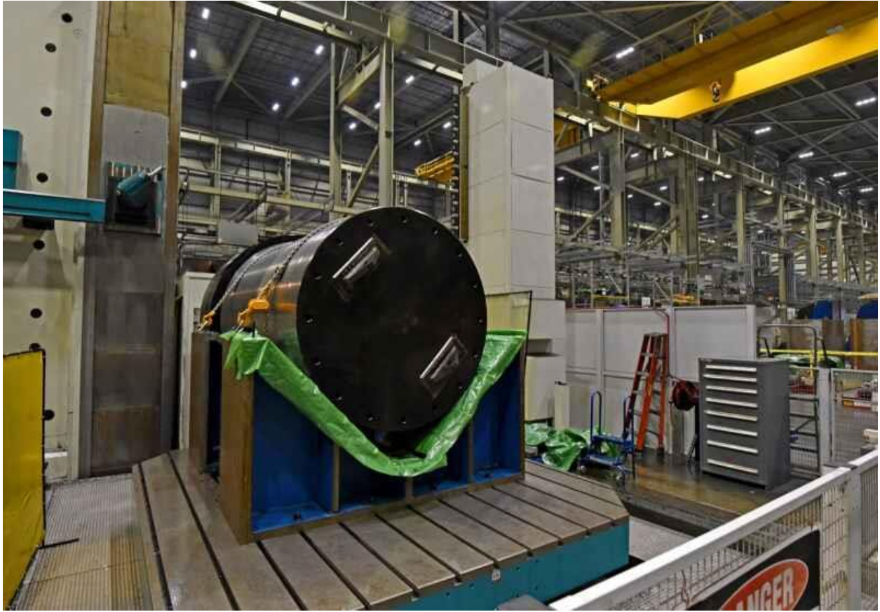
A transport cask in a milling machine at Holtec in Camden, N.J. (April Saul)
