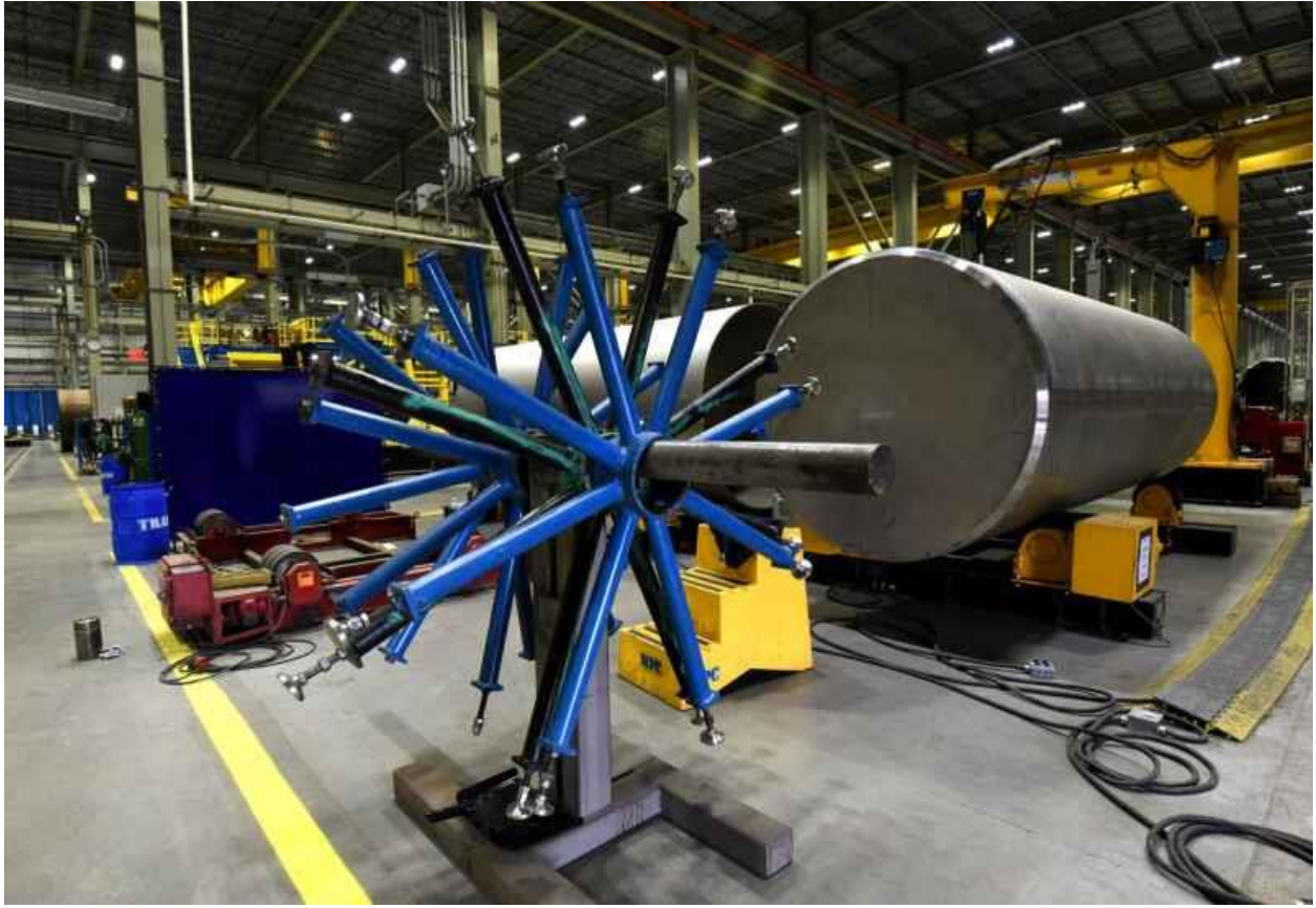
Multi-purpose canister internal spacers at Holtec in Camden, N.J. (April Saul)
