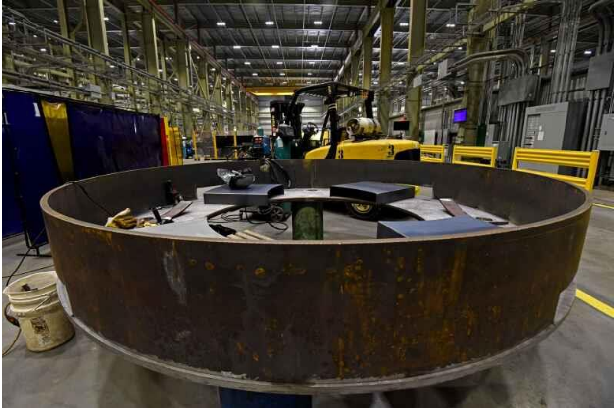
The lower section of a HI-storm overpack in the early fabrication and welding process at Holtec in Camden, N.J. (April Saul)
