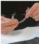
Leave ¾ inch of wire on the end.
