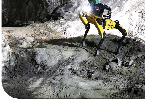
NeBula-SPOT (Networked Belief-aware Perceptual Autonomy robot) undergoing testing inside a cave Credit: NASA/JPL-Caltech
