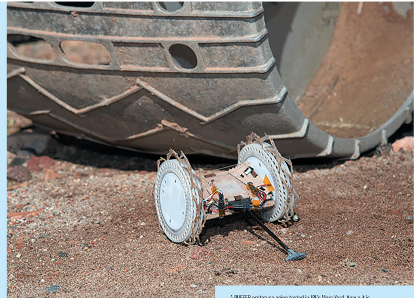
A PUFFER prototype being tested in JPL’s Mars Yard. Above it is a wheel from the Curiosity rover Credit: NASA/JPL-Caltech
