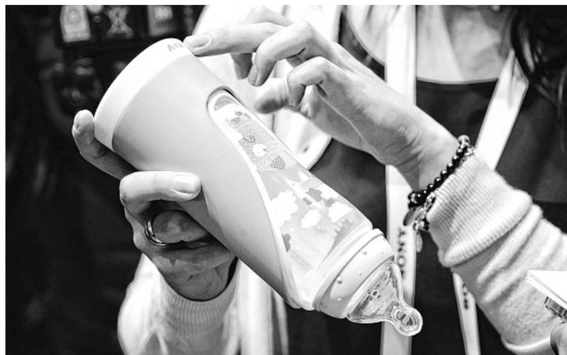
Slow Control smart bottle gives feedback on how to hold it to keep babies from swallowing air.
