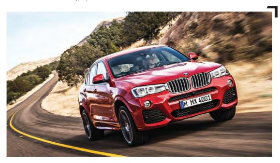
on offer. With a twin turbo six-cylinder of 306hp, it can reach 100 km/h in an exciting 5.5 seconds and has a top end of 247 km/h — this is a fast car that picks up well and can really shift when you, hypothetically of course, put your foot down. She's rock steady at speed, though you'll have to adjust to the breaking distance as it's a little long. It's definitely the kind of car you'll want to get to know before loosening the reigns.
