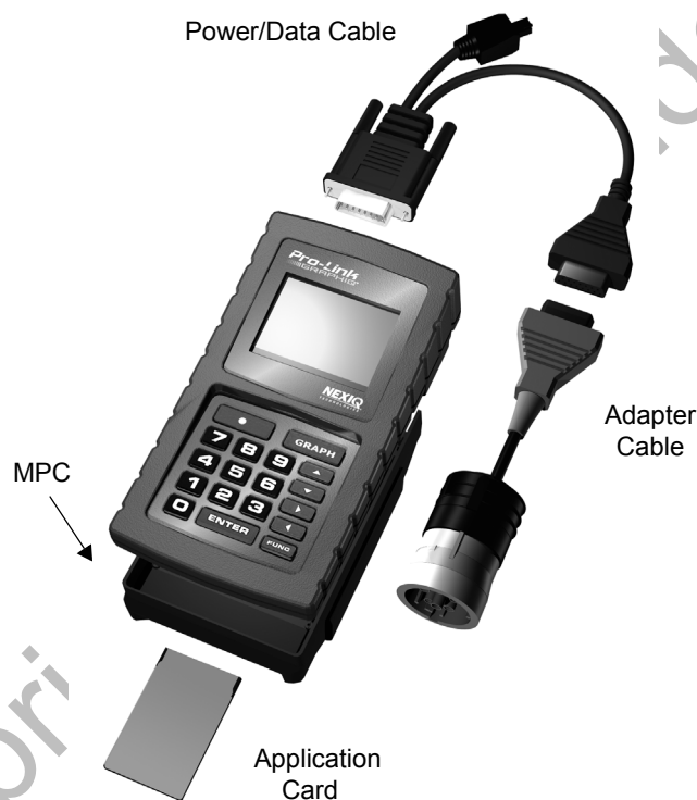
Figure 3.5 Pro-Link GRAPHIQ™ Component Connection
