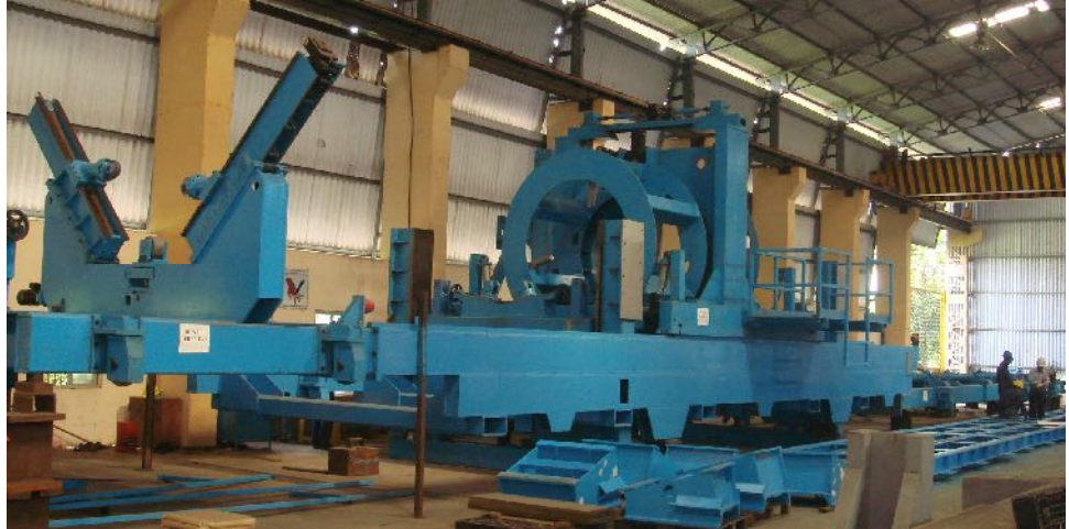
Pipe run-off base frame & equipment
