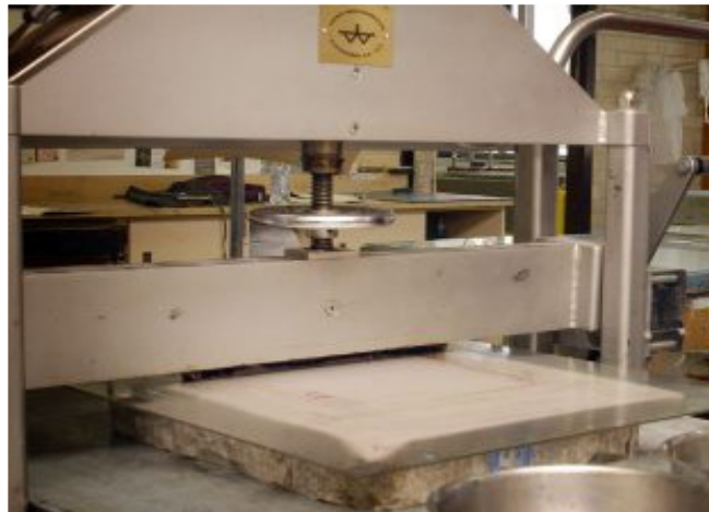
The stone is drawn through the press, and the image is transferred onto the paper.
