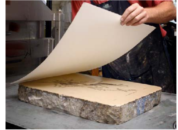
Paper and metal backing are placed onto the image.
