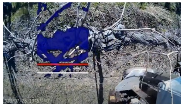
Figure 2: Cabin screen showing LiDAR image and the cutter, which is in the bottom right corner.
