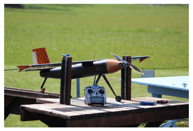
3: Final Aircraft with full fiberglass fuselage
