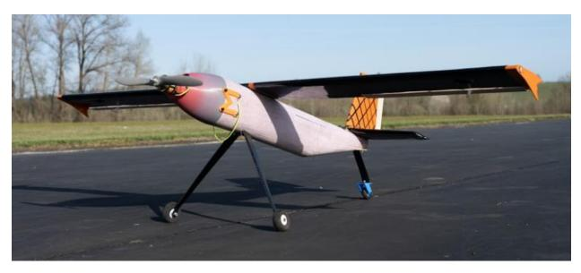
2: Next prototype with carbon fiber wing and landing gear, and symmetrical air foil empennage
