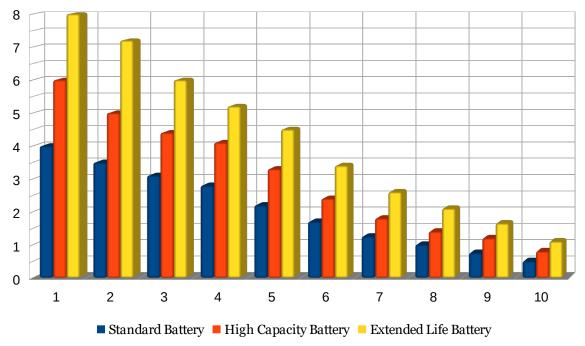
Here you can see that the Extended Life Battery can be used approximately twice as long as the Standard Battery per charge, while the High Capacity Battery is around halfway between the two.
