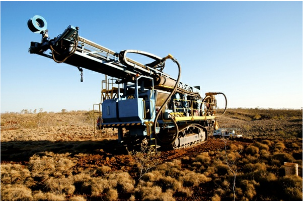
Reverse circulation drill rig. Credit: Thinkstock
